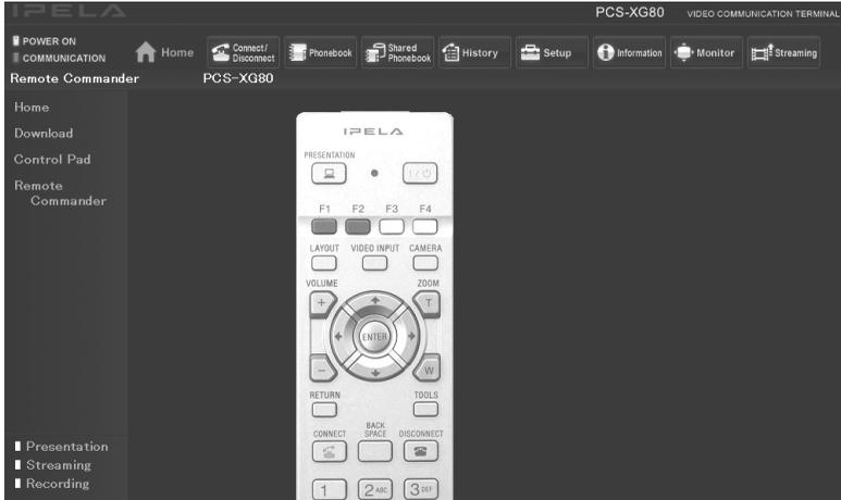
By clicking the various buttons on the Remote Commander image, you can control the system in the same way you can when using a real Remote Commander (PCS-RF1), operating the camera, and dialing phone numbers.
