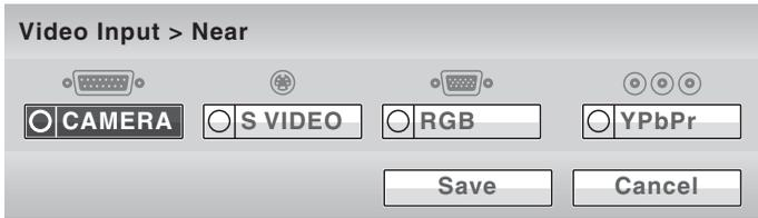
Use the **▲**, **▼**, **◀** or **▶** button on the Remote Commander to select the external equipment connected to each video input on the Communication System, then press the ENTER button.
