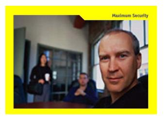
Whether the VSX system is or is not in a call, the video overlay and customized text both appear on the monitor displaying the near-site video, and the customized text alone appears on the screens in the user interface of the near-site system. The far site cannot see the video overlay and customized text on your system.
