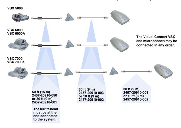
The following diagram shows supported cable configurations for connecting a Visual Concert VSX with a SoundStation VTX 1000 conference phone.
