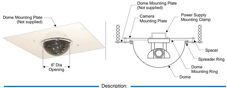
The Ceiling Mount Dome is a lightweight, clear acrylic dome. It can be mounted on most drop ceiling configurations. Telemetrics supplies the dome, dome mounting ring, spreader ring, camera mounting plate, power supply mounting clamp and spacers. Since each ceiling configuration is different, the customer must supply the dome mounting plate or special order it from Telemetrics.
