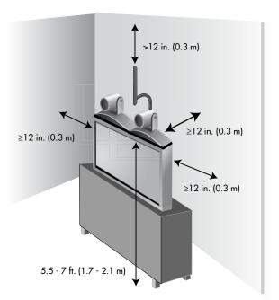
Keep in mind that the camera view is 9 degrees above the line of sight and up to 30 degrees below the line of sight.
