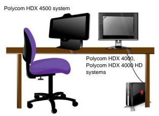
If you need to position one of the Polycom HDX 4000 systems horizontally, remove the stand and install the self-adhesive feet.
