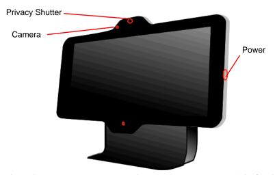
The Polycom HDX 4500 system does not have a separate light for the system. The light on the right side of the monitor indicates power for the monitor and the system.
