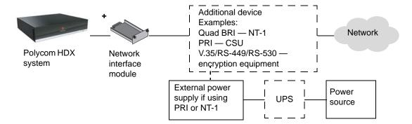
The following diagram shows a general view of how network interface modules are connected with Polycom HDX 8000 series, Polycom HDX 7000 series, and Polycom HDX 4000 series systems.
