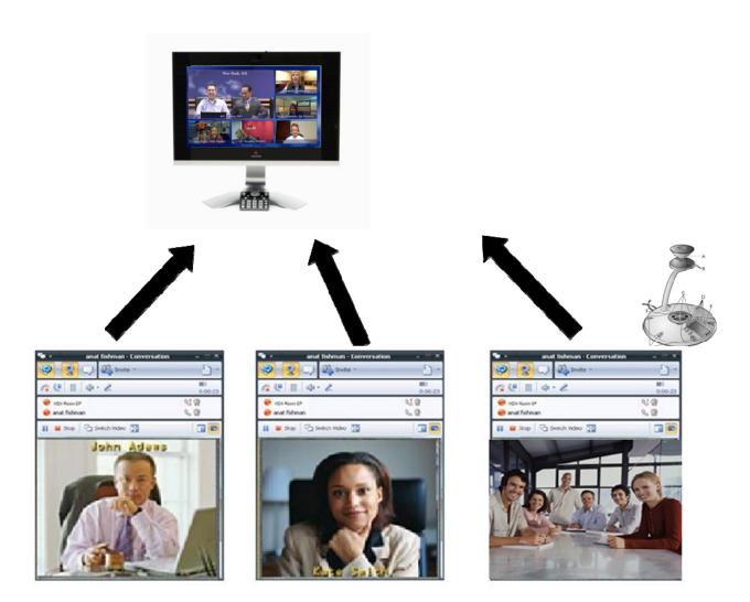
Joe (Office Communicator A) starts a video call with the HDX system (Chardonnay conference room). Jeff (Office Communicator B) starts a video call with the same HDX and so does Mike (Office Communicator C). On the HDX system, the internal MCU is enabled and a multi-point call is established showing all of the participants in a call. If any of the participants are in a room with a CX5000, the view from that room will be the active speaker view.
